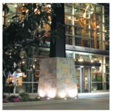
This inground installation grazes the texture of the masonry work, while at the same time guiding the eye upward toward the subject.
