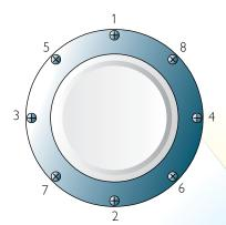
Order in which to tighten screws.
