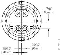
Two (2) 3/4'' NPT threaded conduit inlets
