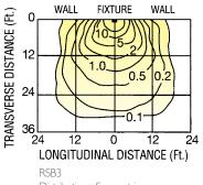
Distribution: Symmetric Lamp/Wattage: 70W HPS Mounting Height: 3' RSC3 – Specular aluminum symmetric.
