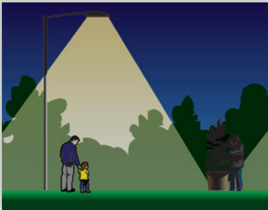
Overhead fixtures project most of their light downward, creating shadows, silhouettes and hot spots.
