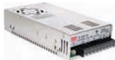
StarStrand 24V 320w Direct Wire Driver 53288 8.5" L x 4.5" W x 2.25" H • 120V/240V input • 24V, 12.5 Amp output • Includes two 72" output cords
