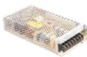
StarStrand 150w Direct Wire Driver 53277 7.75"L x 3.75"W x 1.5"H • 120V/240V input • 12V, 12.5 Amp output • Includes one 72' output cord
